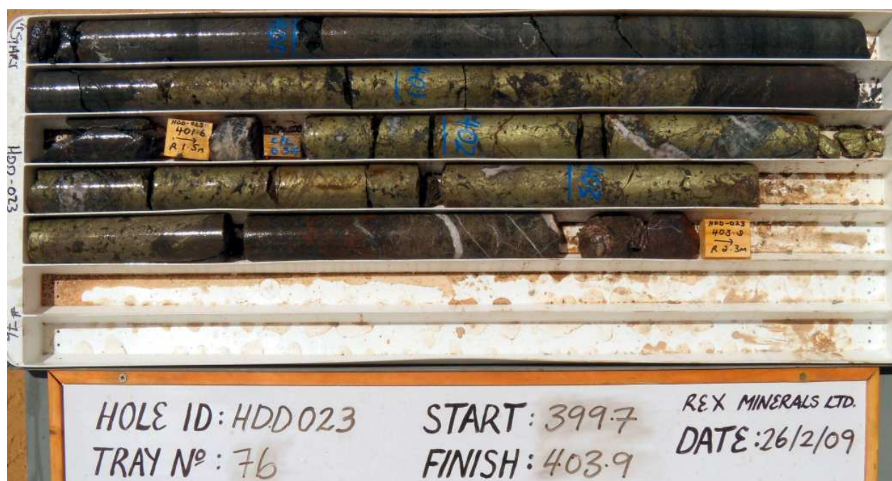
Figure 1: Massive sulphides intersected in drill hole HDD023.
