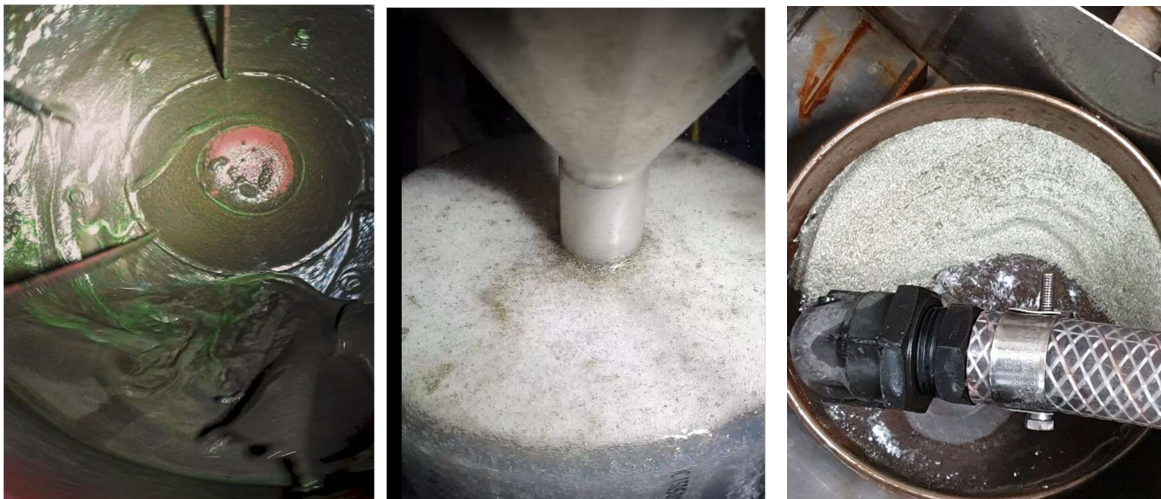
Photo 1 (left): Flotation reagents being added to copper-gold ore
