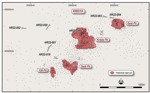
**Figure 1:** Krista plan view RC drill hole relative to the historical Krista and Geib Open Pit mines. Drill Hole HR22-018 was completed underneath the Krista Open Pit.
