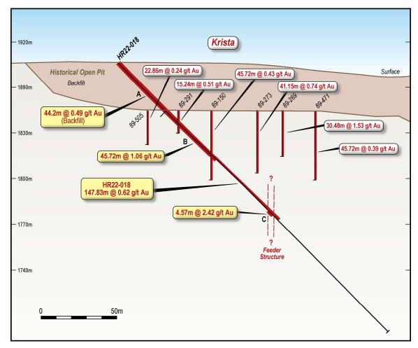
**Figure 2:** Cross Section of HR22-018 shown relative to the shallow and mostly vertical historical RC drilling information. See Figure 1 for the location of drill hole HR22-018.
