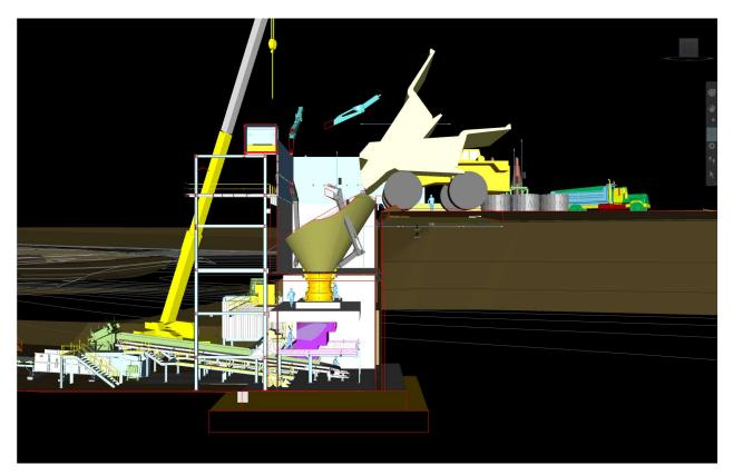
**Figure 3:** Hillside Copper-Gold Project – upgraded jaw-gyratory crusher to allow future direct tip options
