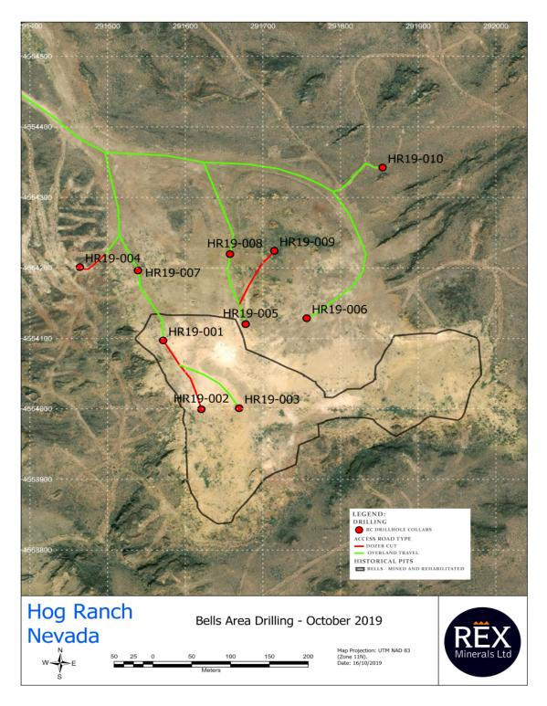
Figure 4: Proposed exploration RC drillhole locations at the Bells Area and access roads
