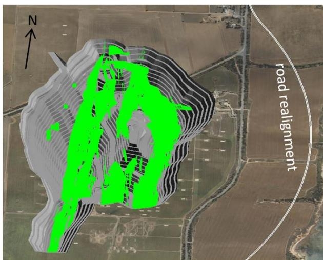
**Figure 2: Copper Ore (green) to be mined from the EFS Pit.**
